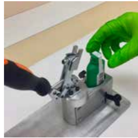
8. Push down on the device until a "click" sound is heard, and the device remains down.
