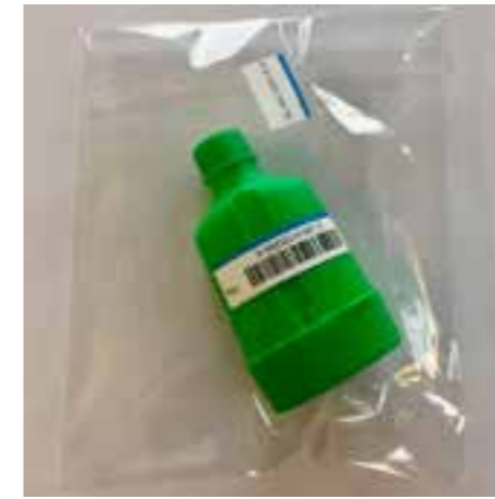
1. BE Sampling Device packaged in a bag that is sealed off with a sample ID label that corresponds to the chain of custody document.
