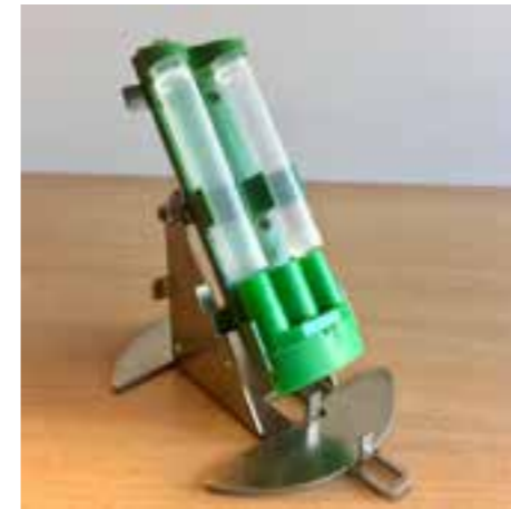
15. Place the mouth piece, including the B&C-sample collectors, in the cradle (in which there are already two plastic test tubes for freeze storage).
