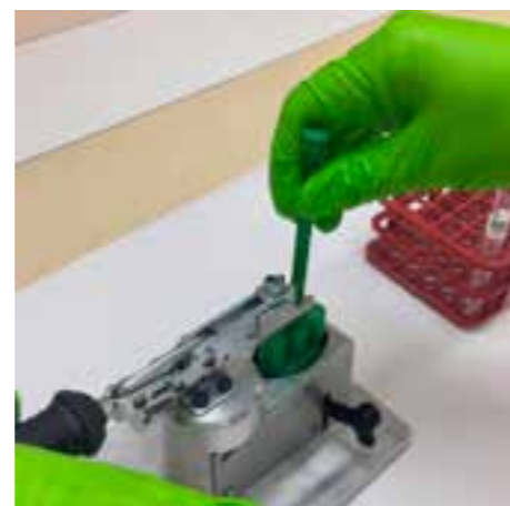
12. Use the handle to push down on the Pick Stick so that it is attached to the collector.
