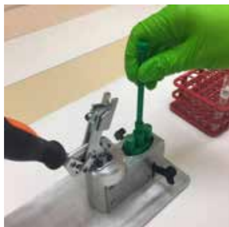
11. Apply the Pick Stick and turn gently until you feel the stick grip to the collector.
