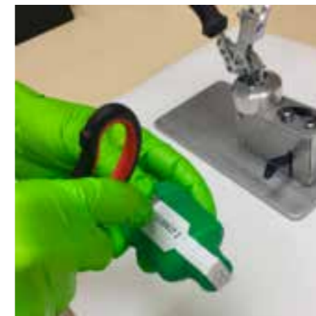
5. If necessary, cut the label along the rim of the large cap that covers the mouth piece.
